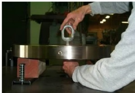
7/8"-14 Lift Eye Attached to Lift Rod #13
