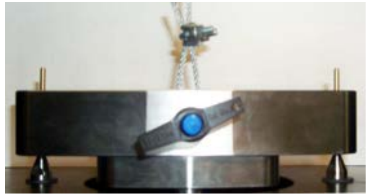
Lowest Yoke Position... Brass Section of Anti-Rotation Pins Fully Visible
