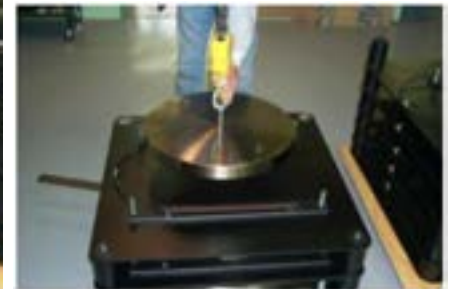
200 LB WT Lowered on to Lifter Pan
