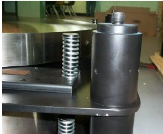
Hand Tighten Spacer & Loosen ¼ Turn
