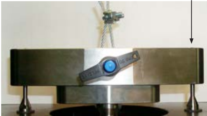
Highest Yoke Position...Top of Yoke Even with Top of Anti-Rotation Pins
