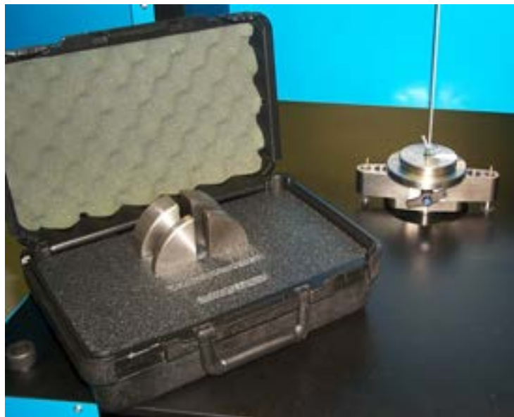
Box for Hand Weights with 1 lbf and 2 lbf Hand Weight Applied to Yoke
