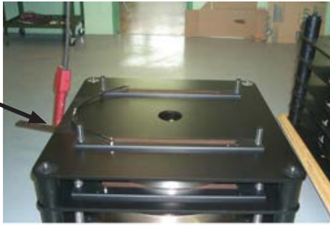
200 LB WT Lowered on to Lifter Pan
