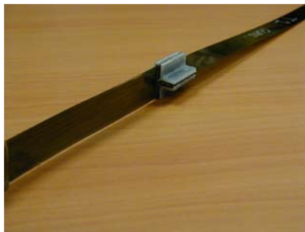
Figure 5. Photograph of the 20 mm width boron tape with 90° joint.
