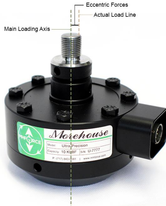
Figure 3: Load Cell showing eccentric forces
