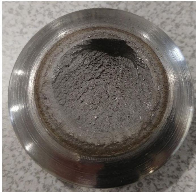
Figure 2: Grade 8 Bolt that Failed at 120,000 lbf and close to 350,000 load cycles
