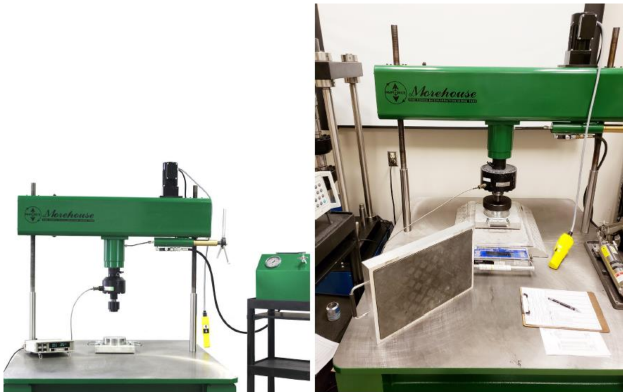
Figure 14: Calibration Adapter for Truck and Aircraft Scales
