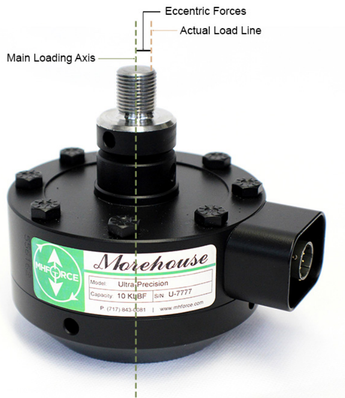
Figure 11: Load Cell Showing Eccentric Forces
