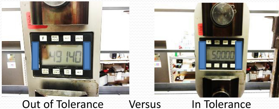
Figure 10: Tension Link Difference in output with pin size
