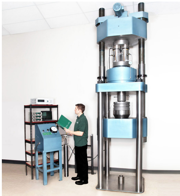
Figure 1: Morehouse Universal Calibrating Machine 1,000,000 lbf Capacity
