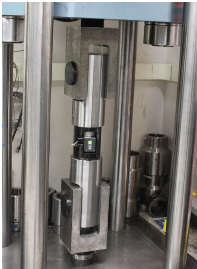
Load Cell Setup with Pins and Clevis
