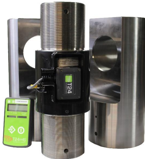
Wireless 300,000 lbf Load Cell with Custom Rod Ends
