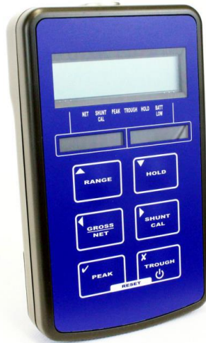
Figure 39: Morehouse PSD Indicator
