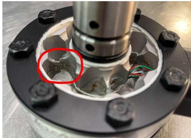
Figure 34: inside an overloaded shear web load cell showing a clear break of the web element.
