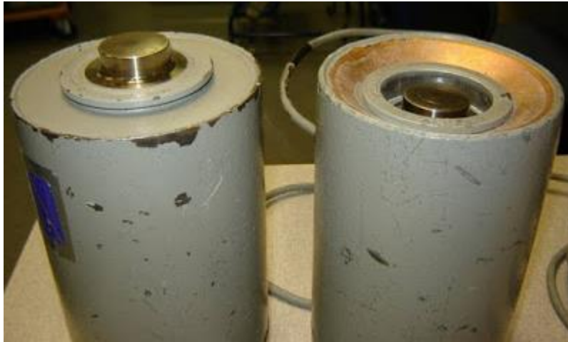
Figure 2: Overloaded Load Cell
