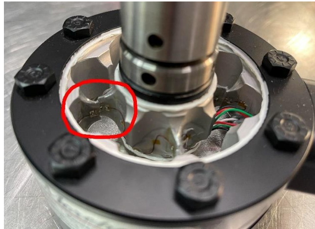
Figure 8: Inside of an overloaded shear web load cell showing a clear beak of the web element
