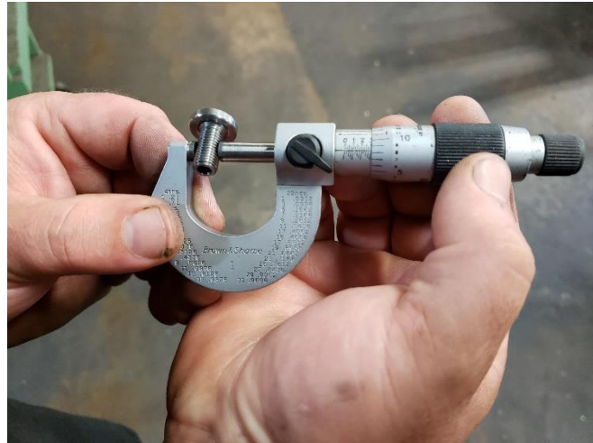
Figure 4: User measuring a part with a micrometer with a resolution of 0.000 1 in.
