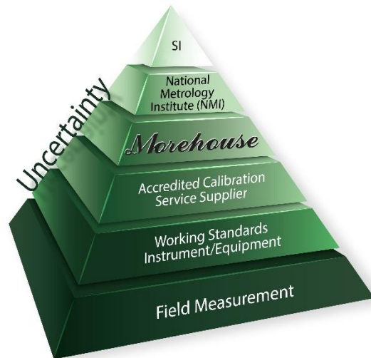
Figure 2: Metrological Traceability Pyramid for Force Measurement
