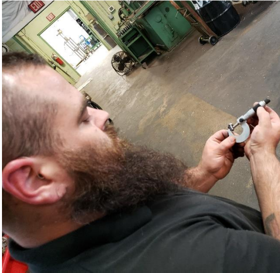
Figure 4: User measuring a part with a micrometer with a resolution of 0.000 1 in.
