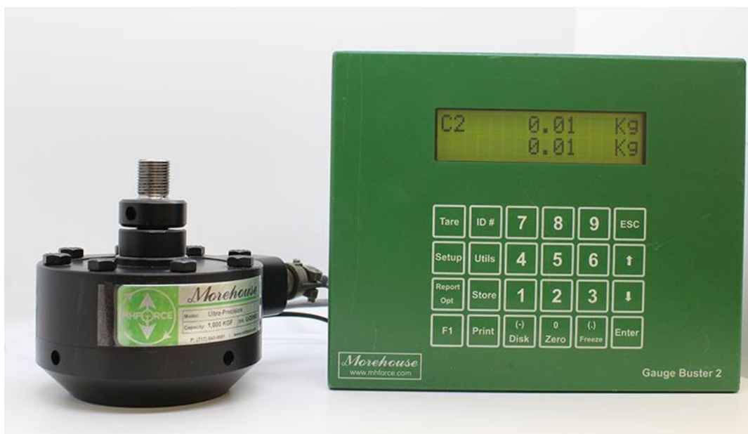
Figure 9: Morehouse Load Cell and Gauge Buster (UUT Example), which is used to Measure Force
