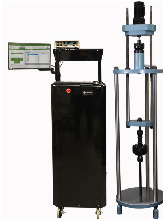
Figure 4: A Morehouse 30K Automation Setup.
