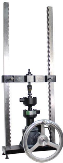
Figure 11. Morehouse BCM Example of Load Cell Calibration
