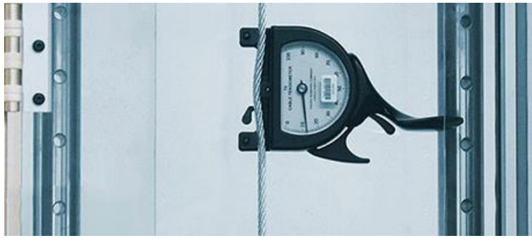
Figure 7. Cable Tensionmeter Calibration
