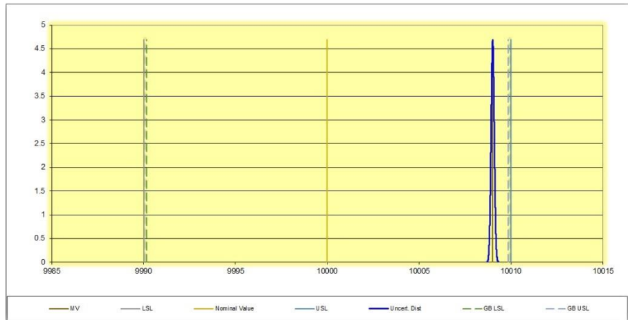
Figure 1: Graph Showing 10 009.0 as the measured value with a 58.789:1 TUR, which is achieved by using a lab with low uncertainties (Morehouse actual example)
