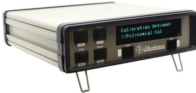
Figure 11: Morehouse 4215 Plus that Uses Coefficients to Reduce Bias
