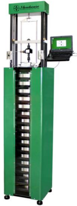
Figure 11 Morehouse 1,000 lbf automated deadweight machine
