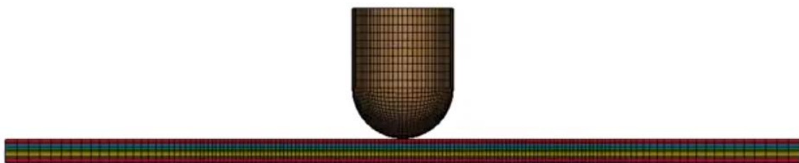
Fig.1. Meshed model of PALF/Epoxy composite laminate with hemispherical impactor
