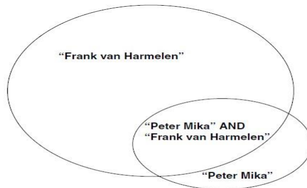
Figure 3.4. The Jaccard-coefficient does not show a correlation in cases where there is a significant difference in the sizes of the two sets such as in the case of a student and a professor.
