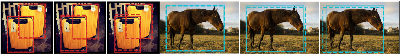
Figure 1. Example results from COCO validation using Mask R-CNN [2] trained using (left to right) \mathcal{L}_{GIoU} , \mathcal{L}_{IoU} , \ell_1 -smooth losses. Ground truth is shown by a solid line and predictions are represented with dashed lines.
