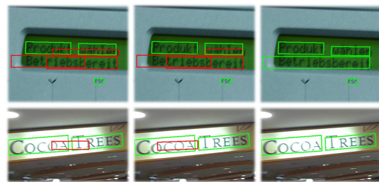
Figure 6. Three steps in Recalled NMS. Left: results of traditional NMS (quadrilaterals in red are false detection). Middle: recalled high score quadrilaterals. Right: merging results by closeness.
