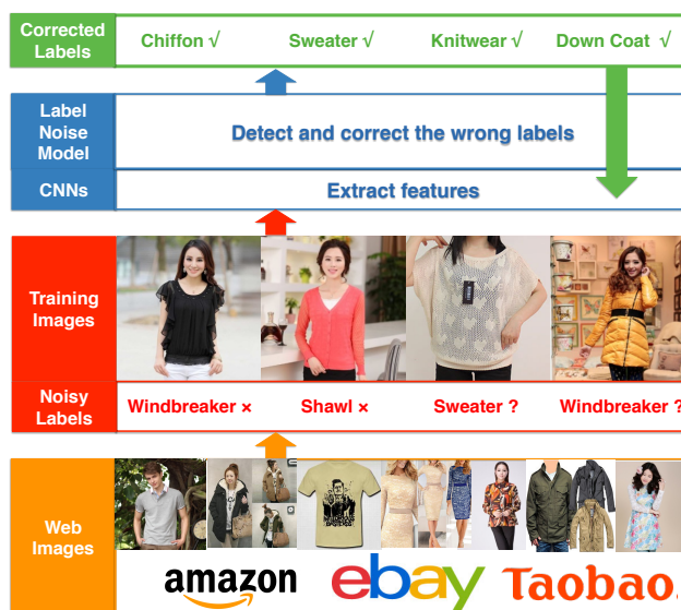
Figure 1. Overview of our approach. Labels of web images often suffer from different types of noise. A label noise model is proposed to detect and correct the wrong labels. The corrected labels are used to train underlying CNNs.
