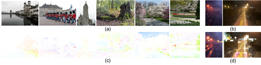
Figure 2. (a) Example images in our daytime haze-free image database. (b) Nighttime haze images. (c) The maximum reflectance maps of (a). (d) The Maximum reflectance maps of (b).
