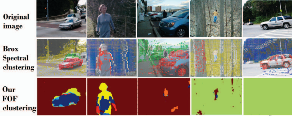
Figure 4. Comparison of segmentation algorithms. The rows correspond to the original images, spectral clustering [13], and our FOF segmentation. The tracked keypoints used in spectral clustering are shown as squares with their colors representing the cluster memberships. Despite the use of a post-processing merge step in the implementation, in many images, spectral clustering is not certain about some background keypoints (white squares) and in cases with large depth disparity, the background is broken into smaller sections. Our method avoids these errors and also results in a dense labeling of the image. The last column is an example of our method failing because the car happens to move consistently with the FOF due to camera motion. More comparisons are provided in the supplementary submission.
