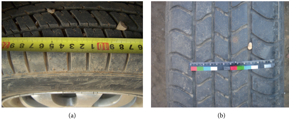
FIGURE 4: Application of tyre inclusion identification. (a) Tyre #1. (b) Tyre #2.
