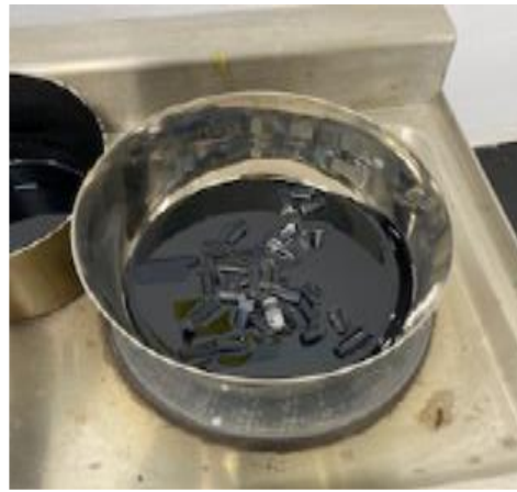
Figure 12. Heating the polymers with the heated bitumen
