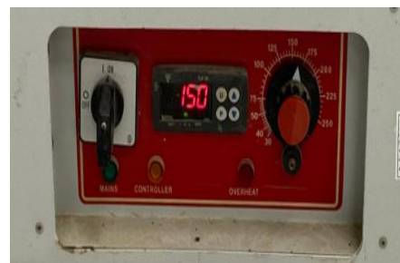
Figure 19. Putting the mould in the drying oven at 155°C
