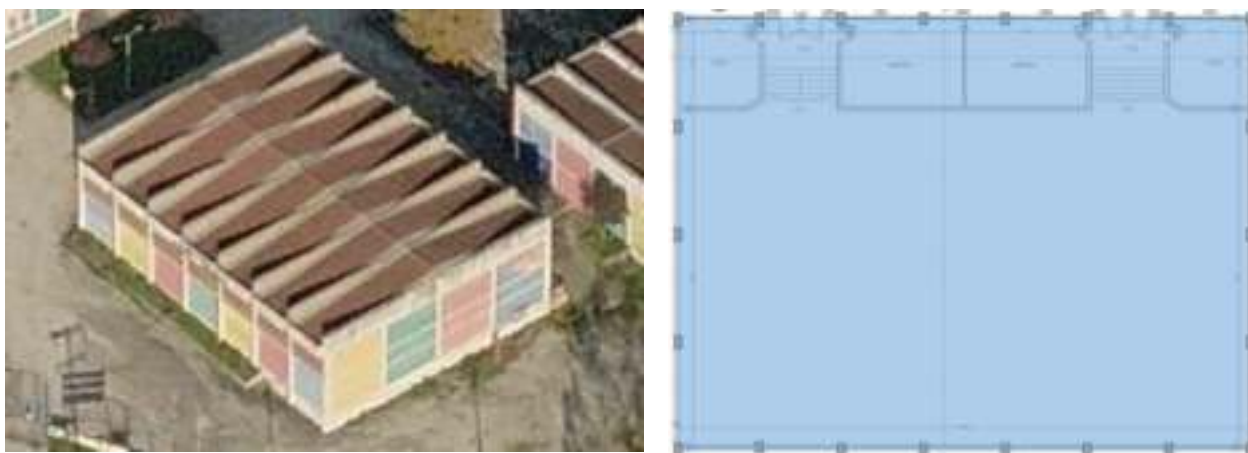
Figure 29 The Sports Hall building a) aerial view (left) and b) sketch of the heated floor area (right)
