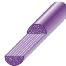
Polytron with fiberglass the length of the pellet (not to scale)
