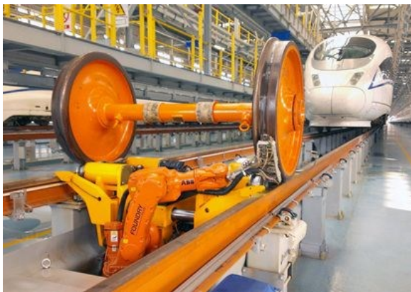
UW-UT system on a calibration reference wheelset (left) and an on-vehicle wheelset inspection (right).
