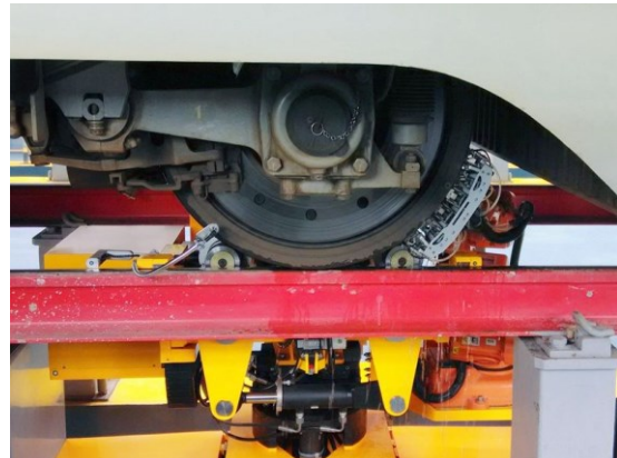
UW-UT system on a calibration reference wheelset (left) and an on-vehicle wheelset inspection (right).
