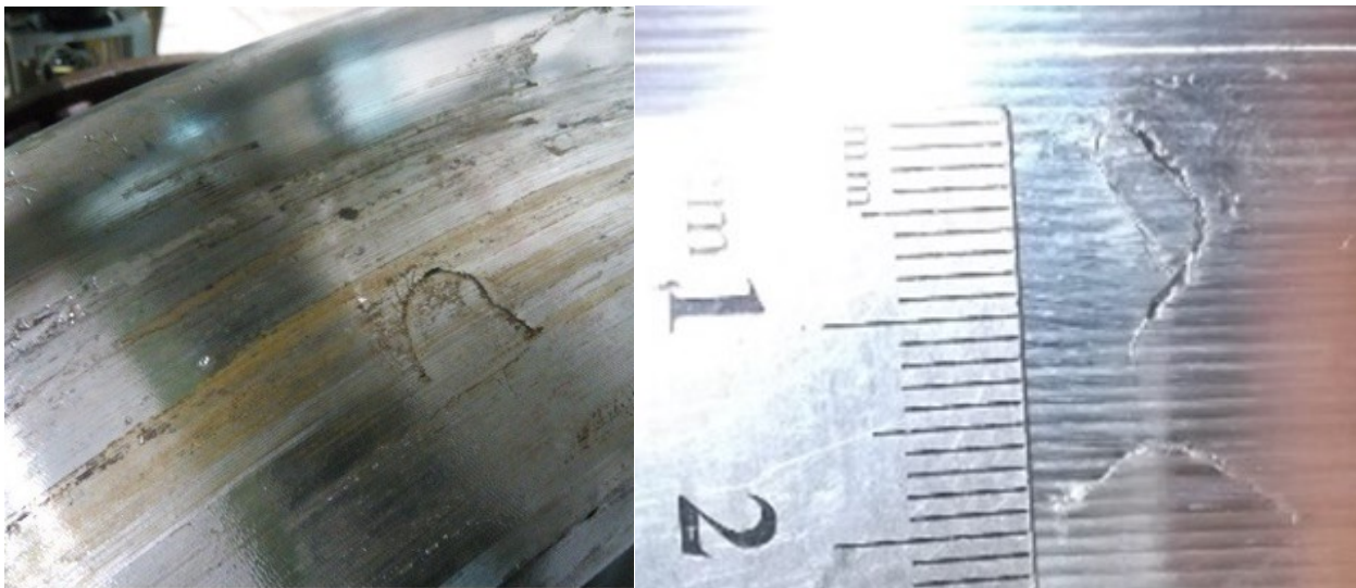
Wheel fatigue crack findings (left) before and (right) after tread reprofiled
