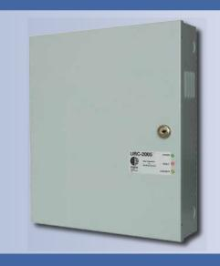
The URC-2000 Universal Controller allows control of two access control points (doors). It utilizes flash firmware for easy upgrades, and employs fully distributed intelligence for off-line operations. Decisions such as access level changes, schedule activation and card expiration are made by the URC-2000 controller without the need of a computer.
