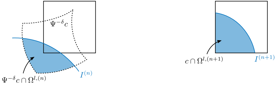
(a) The dashed curves correspond to the boundary of the preimage of c , which is denoted by \Psi^{-\delta}c . The solid curve corresponds to the fluid interface I^{(n)} and the shaded region corresponds to \Psi^{-\delta}c \cap \Omega^{l,(n)} (cf. the right-hand side of eq. (3)).
