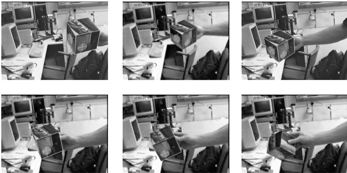
Figure 7.8: Images from a sequence when the object is rotating and the parts of the object which are self-occluded changes mid-sequence. Also, the hand occludes part of the object during the sequence but the performance of the tracker is not affected.
