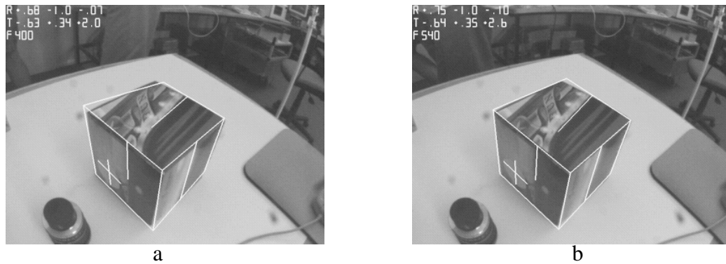
Figure 7.11: Perspective Camera with Zoom Model: The (a) first and (b) 75 th images from a sequence where the incorrect initial focal length of 400 pixels changes to the correct value of 550 pixels. The pose parameters and focal length are shown in the top left hand corner of the images. Note how in image (b) the projected outline fits the object unlike image (a).
