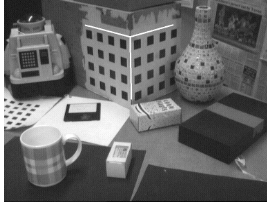
Figure 5.15: The orthogonal triad of angles on the calibration object (highlighted) which are measured in the metric reconstruction from sequence I, and compared to the veridical values of 90^\circ . The angles are measured between the planes of calibration grid, and the planes are fitted by orthogonal regression to 23 and 18 points on the left and right grids, and 15 points on the top row.
