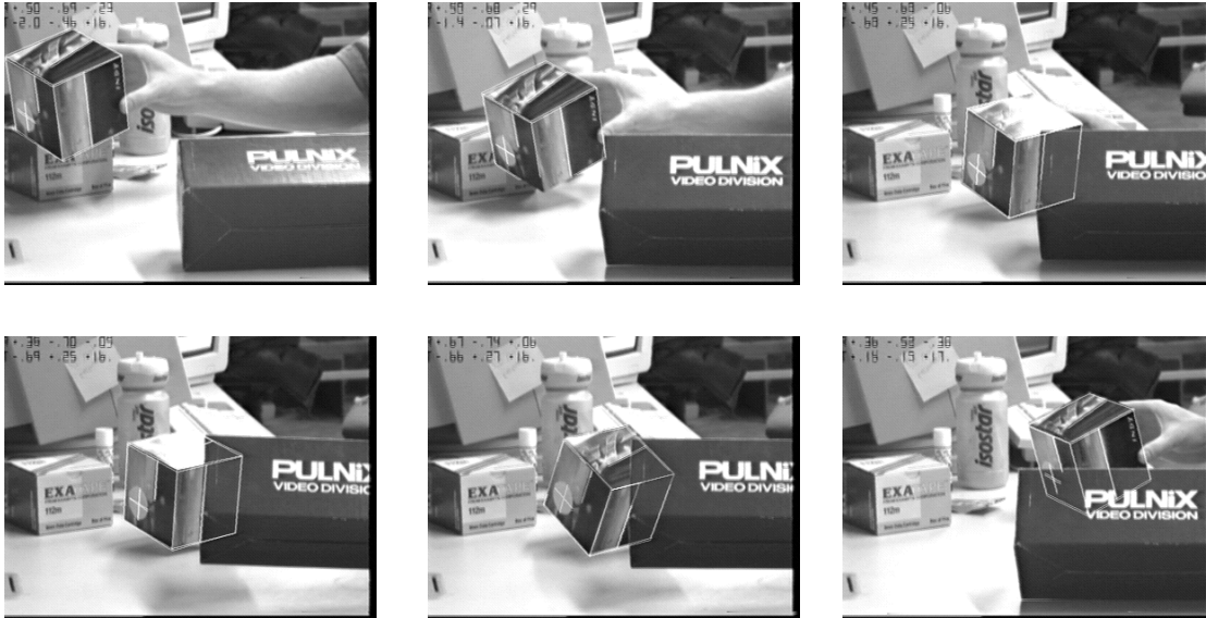
Figure 7.6: Images from a sequence when the object is partially occluded, but the robust tracker remains locked onto the object. Note, both internal (texture) and external (occluding) boundaries are tracked. The cross marks a tracked ellipse.
