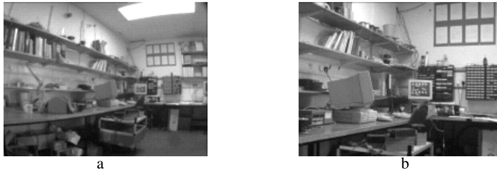
Figure 2.2: (a) The radial distortion affect with a short focal length camera. Note that lines straight in the scene are not necessarily straight in the image. (b) The same scene viewed with a longer focal length lens.
