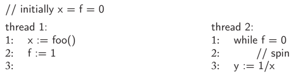
Figure 2.5: A simple example of flag-based synchronization. To avoid a spurious error, the update to x must be visible to thread 2 before the update to f .
