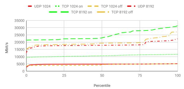
UDP versus TCP with Stateless Offloads On/Off; 1024 and 8192 bytes per send/packet
