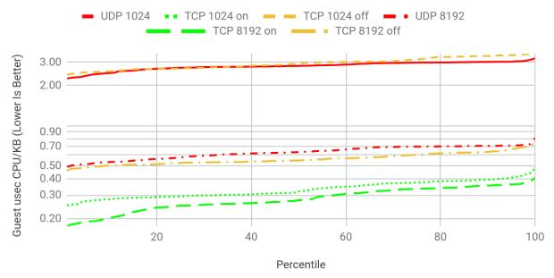
Again, we can see how either larger packets on the wire, or the stateless offloads (TSO/GSO, LRO/GRO) greatly improve the per-unit cost of data transfer.
