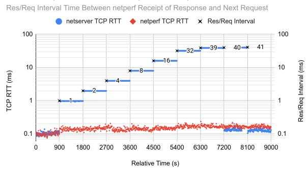
TCP Computed RTT vs Response/Request Interval
