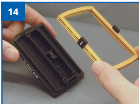
14 Once the superglue has dried, place the frame over the raised ridge on the underside of the platform.
