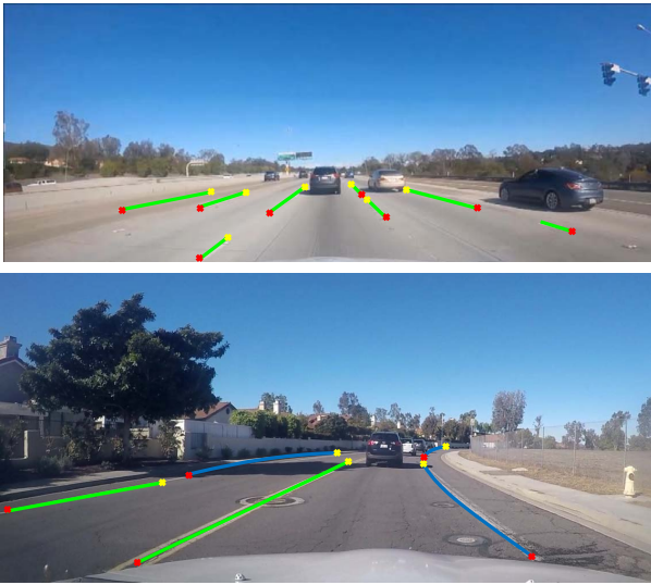
Figure 5: Exemplar results of lane detections. We detected both straight lanes (red) and curved lanes (blue).
