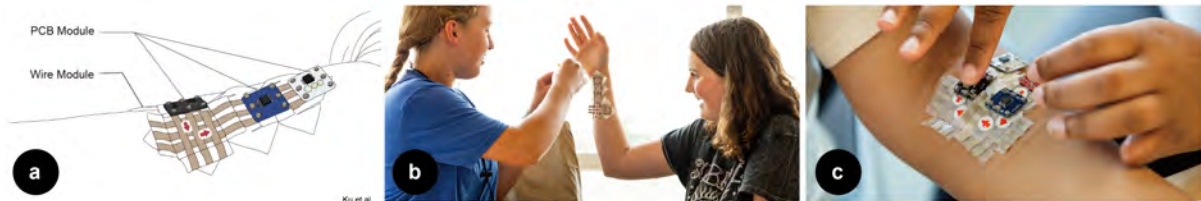
Figure 1: This paper investigates using an on-skin toolkit, SkinKit [22], in a hands-on workshop designed for middle school students. (a) The SkinKit device consists of PCB modules and skin-conformable wire modules. (b) Students worked in pairs. (c) Students experienced prototyping different wearable functionalities and designed the look and placement on the body.
