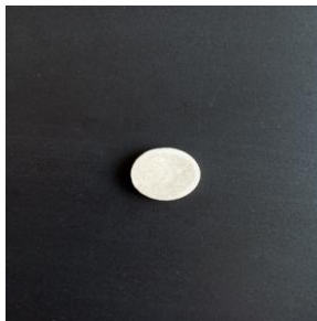
Fig.1. The sample of a ceramic target from doped with Sn BaTiO 3 gel powders.
