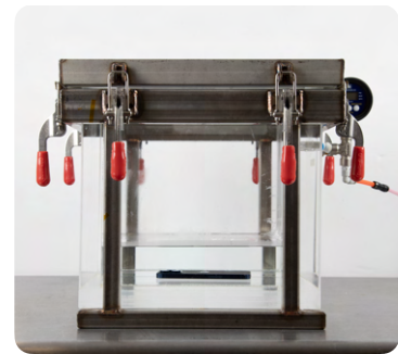
To test for IPX7/8 water immersion protection, Apple submerges iPhone inside a pressurized vessel to simulate pressure experienced underwater.
