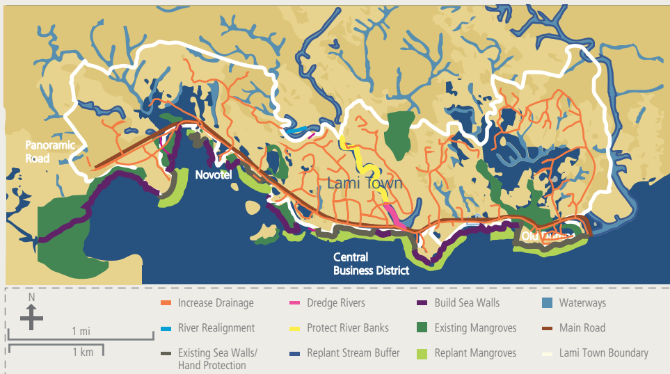
A map of Lami Town, Fiji, showing a mix of the conventional engineering and ecosystem options identified and evaluated by the team © UN-Habitat 2014c
