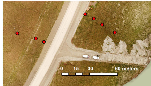
Figure A1. Transect of iButton soil temperature loggers across the Dalton highway at our site close to Deadhorse ( 70.099^\circ\text{N} , 148.511^\circ\text{W} ). Red dots indicate the position of iButton sensors, the bright grey element shows the gravel road surface, the adjacent darker grey elements show the road shoulders. To the right a side road leading to the adjacent Sagavanirktok River (lower right) is seen (drone photo by Soraya Kaiser).
