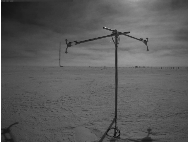
Figure 1. Spectral albedo measurement at Dome C (picture taken on 12 January 2014, 11:00 LT). The vertical mast is approximately 2 m high.
