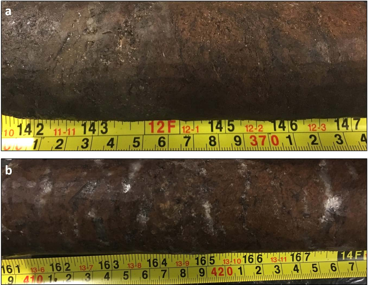
1004 Figure 9: (a) Stratigraphic contact between the base of the frozen silt and peat layer occurring at 1005 3.65 m and the underlying frozen peat. (b) Example of organic-matrix microlenticular to 1006 suspended cryostructures developed in the peat below the stratigraphic contact shown in (a).
