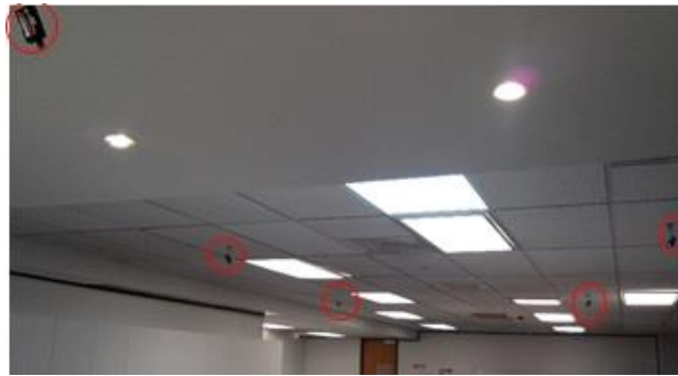
Figure 4. Physical deployment of 14 XM1000 motes in the research lab
