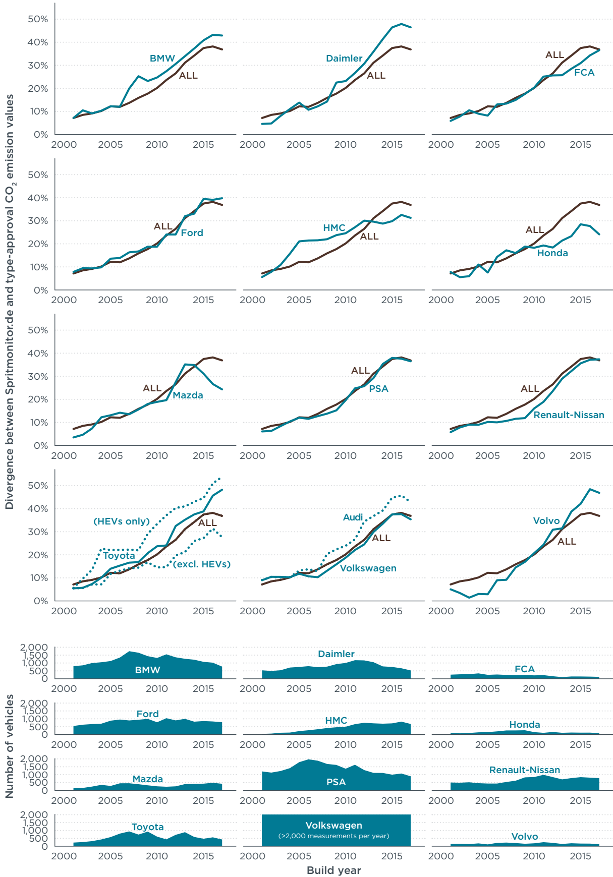
Figure 9. Divergence between Spritmonitor.de and type-approval CO 2 emission values by manufacturer group. The bottom graphs display the number of vehicles per manufacturer group and build year.
