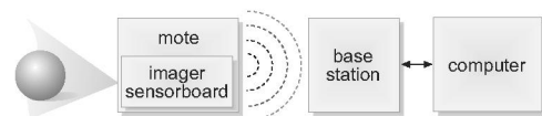
Fig. 1. System overview: WSN node (mote) with ALOHA sensorboard streams captured images to a base node connected to a PC.
