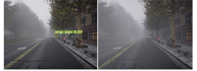
Figure 12: Stop sign can be detected in light fog, while a FP case occurs in dense fog.
