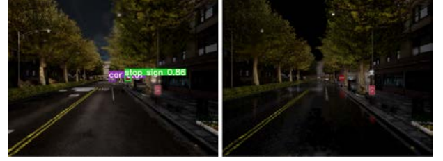
Figure 11: Stop sign can be detected in light rain, while a FP case occurs in heavy rain.
