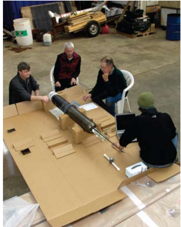
Figure 3. Pre-cruise diagnostic testing of a US Argo SOLO float in Wellington, New Zealand. Photo by Alan Blacklock, NIWA, NZ
