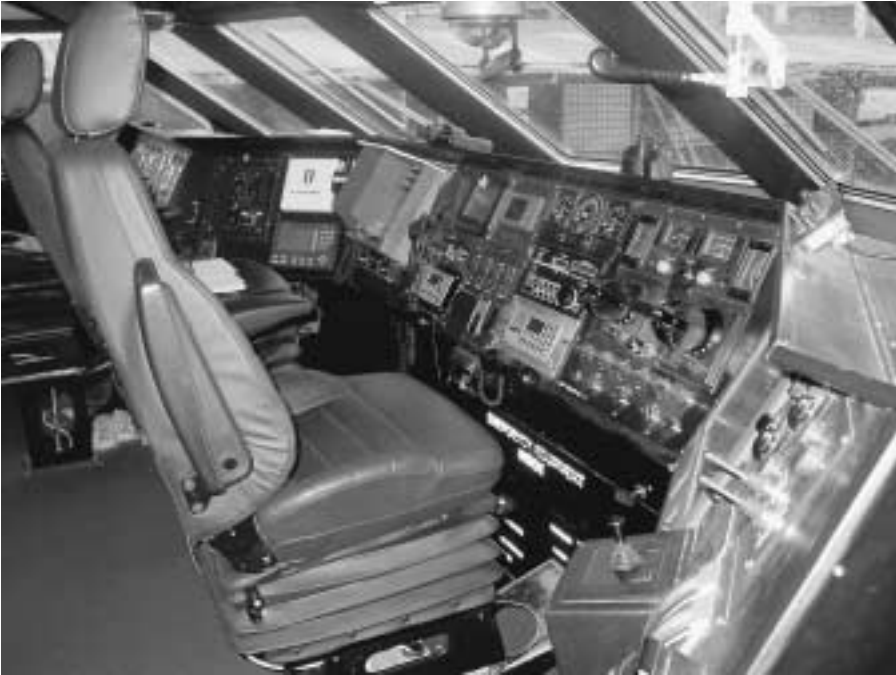
FIGURE 2-3 Wheelhouse of the Victoria Clipper , a high-speed ferry. (Photo courtesy of David Natali, Clipper Navigation, Inc.)
