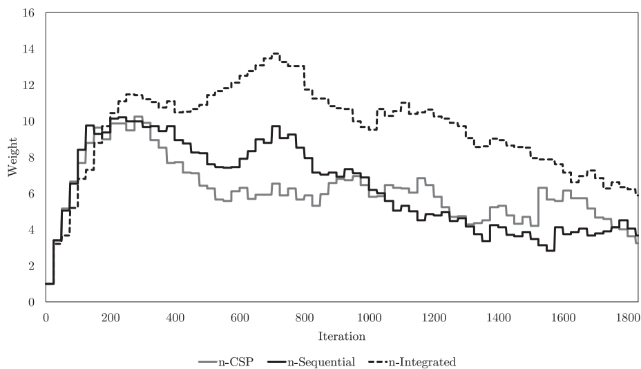
Fig. 7. Performance of neighborhoods for instance SE1_5 when the ALNS heuristic is initialized with the line solution. The iteration number is shown on the x-axis and the weight of the neighborhoods is shown on the y-axis. The weight is calculated based on Equation (17). The score parameters \psi_1 and \psi_2 are 25 and 0, respectively.
