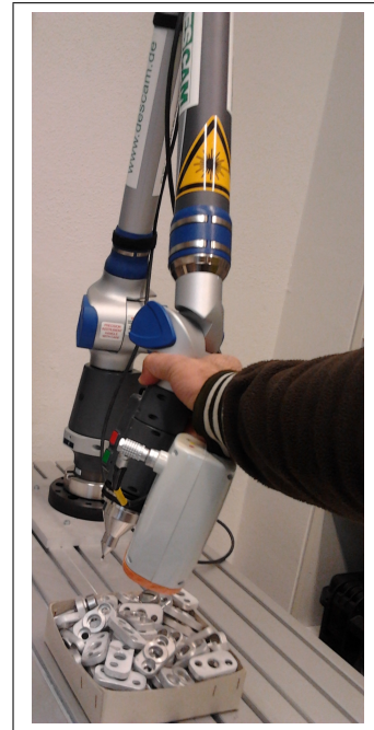
Figure 1: Laser Scanner ModelMaker D100: Scanning Scenario
