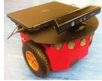
Figure 14. Microsoft Kinect mounted on Pioneer P3-DX mobile robot.
